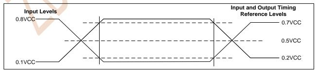
Figure 8.3 AC Measurement I/O Waveform
