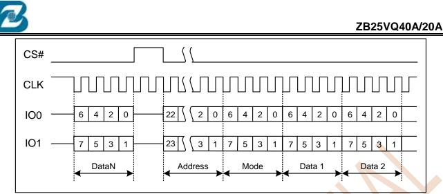
Figure 7.18 Fast Read Dual I/O Instruction (Initial command or previous M5-4=10)
