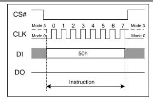
Figure 7.3 Write Enable for Volatile Status Register Instruction
