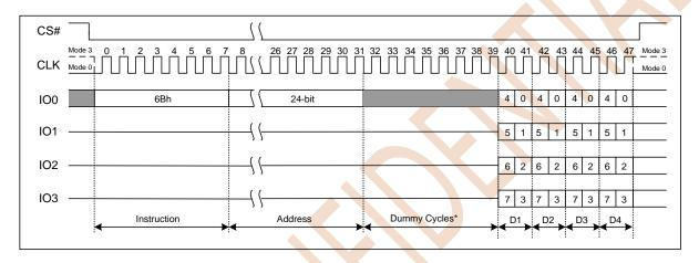
Figure 7.16 Fast Read Quad Output Instruction
