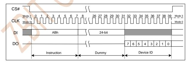
Figure 7.25 Release Power-down / Device ID
