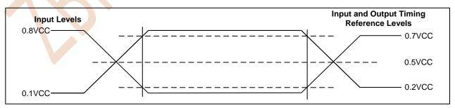
Figure 8.3 AC Measurement I/O Waveform
