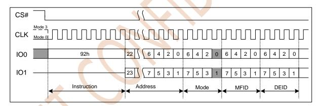
Figure 7.29 Read Manufacturer/Device ID Dual I/O Instruction
