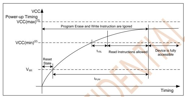
Figure 8.1 Power-up Timing
