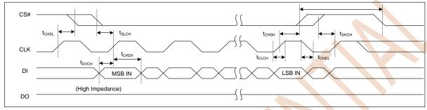
Figure 8.5 Input Timing
