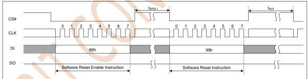
Figure 8.7 Software Reset Input Timing
