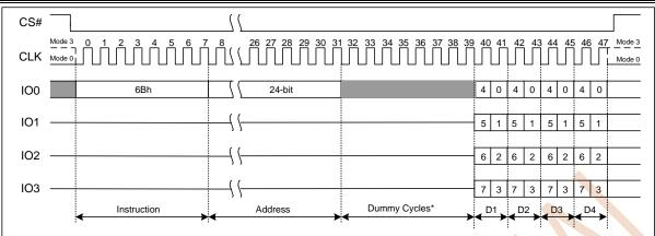
Figure 7.16 Fast Read Quad Output Instruction
