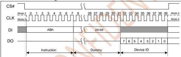
Figure 7.29 Release Power-down / Device ID
