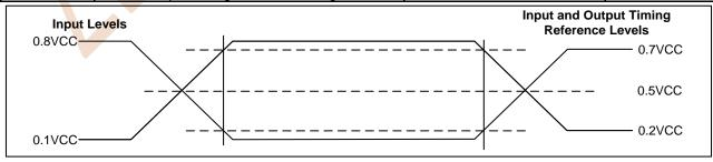
Figure 8.3 AC Measurement I/O Waveform
