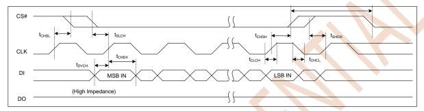
Figure 8.5 Input Timing
