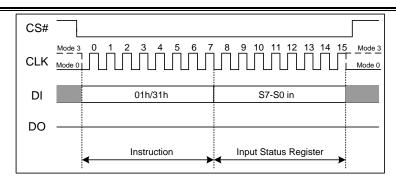
Figure 7.5 Write Status Register Instruction(SPI Mode)
