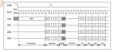
Figure 7.19 Fast Read Quad I/O Instruction(Initial command or previous M5-4 \neq 10)
