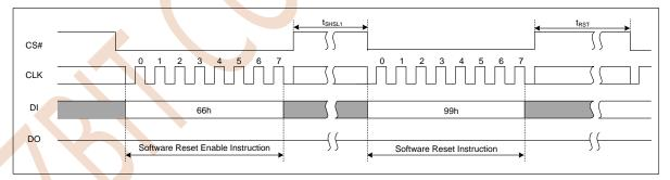
Figure 8.7 Software Reset Input Timing
