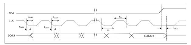
Figure 8.4 Serial Output Timing
