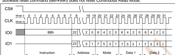
Software reset command (66h+99h) does not reset Continuous Read Mode.
