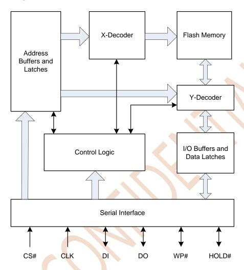
Figure 2.1 Block Diagram
