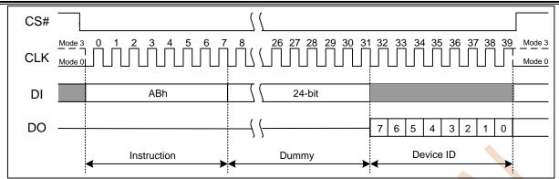
Figure 7.25 Release Power-down / Device ID
