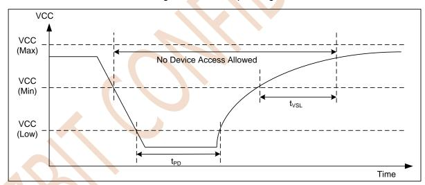
Figure 8.2 Power-Down and Voltage Drop
