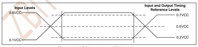
Figure 8.3 AC Measurement I/O Waveform
