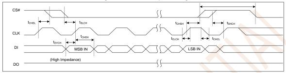
Figure 8.5 Input Timing
