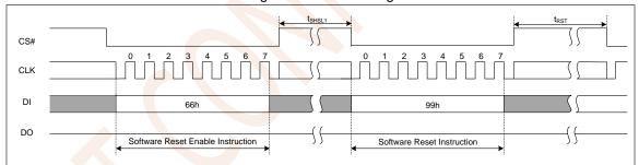
Figure 8.7 Software Reset Input Timing
