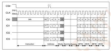
Figure 7.32 Read Manufacturer/Device ID Quad I/O Instruction
