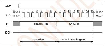
Figure 7.5a Write Status Register Instruction(SPI Mode)
