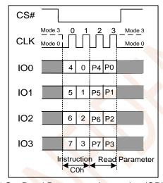
Figure 7.34 Set Read Parameters Instruction (QPI Mode only)
