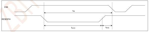
Figure 8.8 Hardware Reset Timing
