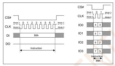
Figure 7.22 Deep Power-down Instruction(SPI and QPI Mode)
