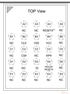
Figure 3.4 24-BALL TFBGA (5x5 ball array)
