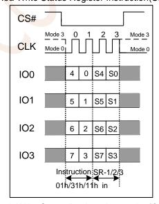
Figure 7.5b Write Status Register Instruction(QPI Mode)
