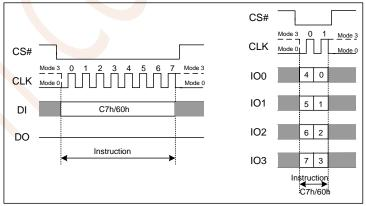
Figure 7.10 Chip Erase Instruction(SPI or QPI Mode)
