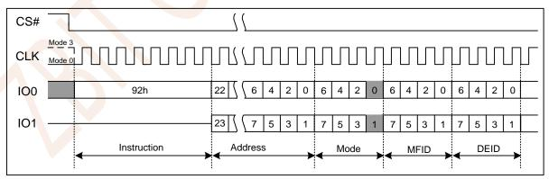
Figure 7.31 Read Manufacturer/Device ID Dual I/O Instruction
