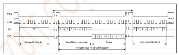
Figure 7.11a Erase / Program Suspend Instruction(SPI Mode)
