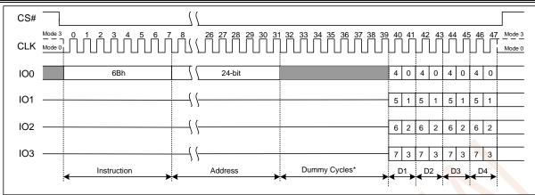
Figure 7.16 Fast Read Quad Output Instruction
