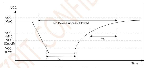
Figure 8.2 Power-Down and Voltage Drop
