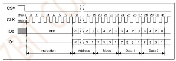
Figure 7.17 Fast Read Dual I/O Instruction (Initial command or previous M5-4\neq 10)
