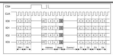
Figure 7.19b Fast Read Quad I/O Instruction(Previous command set M5-4 = 10)
