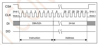
Figure 7.9a Block Erase Instruction(SPI Mode)
