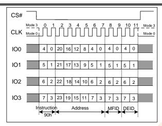
Figure 7.25b Read Manufacturer/Device ID(QPI Mode)
