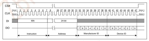
Figure 7.25a Read Manufacturer/Device ID(SPI Mode)
