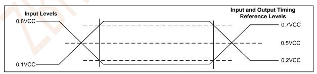
Figure 8.3 AC Measurement I/O Waveform
