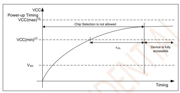
Figure 8.1 Power-up Timing
