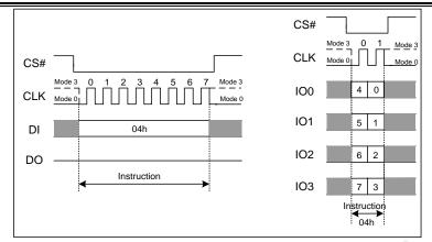
Figure 7.4 Write Disable Instruction(SPI or QPI Mode)
