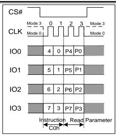
Figure 7.44 Set Read Parameters Instruction (QPI Mode only)
