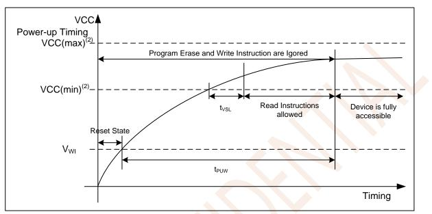
Figure 8.1 Power-up Timing
