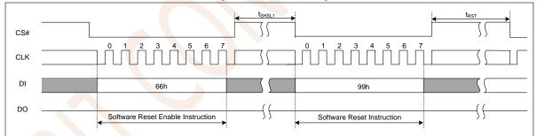
Figure 8.7 Reset Input Timing
