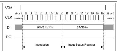
Figure 7.5a Write Status Register Instruction(SPI Mode)
