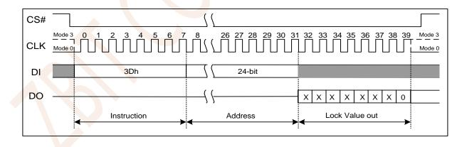
Figure 7.38a Read Block Lock Instruction(SPI Mode)
