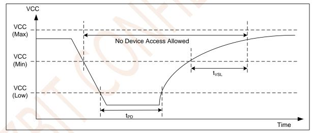
Figure 8.2 Power-Down and Voltage Drop
