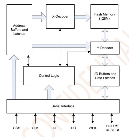
Figure 2.1 Block Diagram
