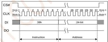
Figure 7.37a Individual Block/Sector Unlock Instruction(SPI Mode)
