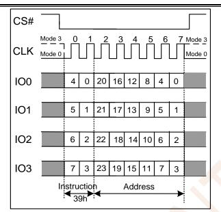
Figure 7.37b Individual Block/Sector Unlock Instruction(QPI Mode)
