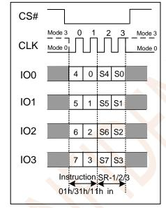
Figure 7.5b Write Status Register Instruction(QPI Mode)
