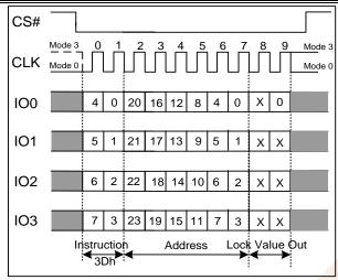
Figure 7.38b Read Block Lock Instruction(QPI Mode)
