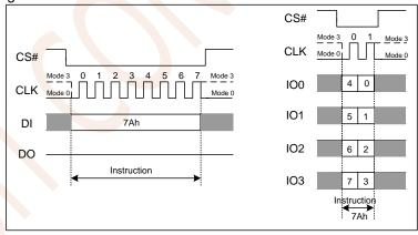
Figure 7.12 Erase/Program Resume Instruction(SPI or QPI Mode)
