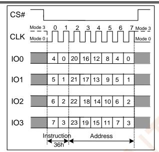
Figure 7.36b Individual Block/Sector Lock Instruction(QPI Mode)
