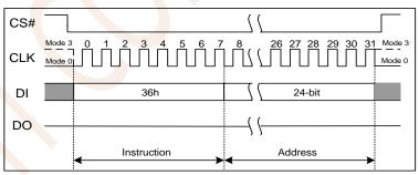
Figure 7.36a Individual Block/Sector Lock Instruction(SPI Mode)
