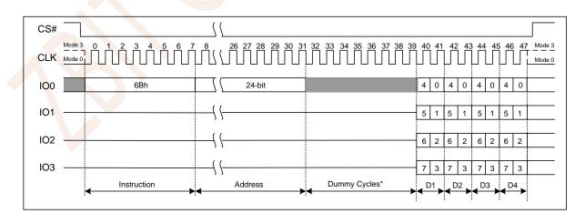
Figure 7.16 Fast Read Quad Output Instruction
