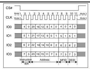
Figure 7.30b Read Manufacturer/Device ID(QPI Mode)
