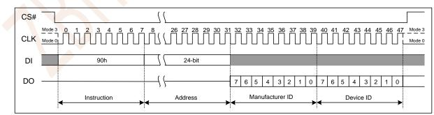
Figure 7.30a Read Manufacturer/Device ID(SPI Mode)
