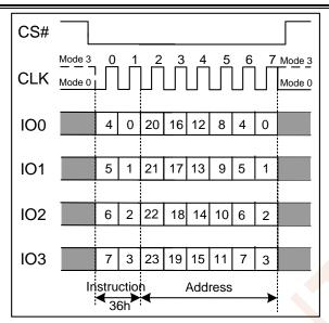
Figure 7.34b Individual Block/Sector Lock Instruction(QPI Mode)
