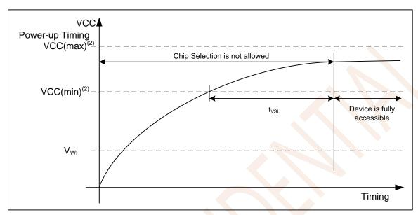
Figure 8.1 Power-up Timing
