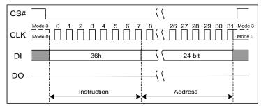
Figure 7.34a Individual Block/Sector Lock Instruction(SPI Mode)
