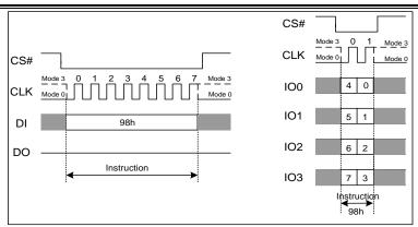
Figure 7.38 Global Block Lock Instruction(SPI or QPI Mode)
