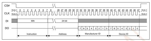
Figure 7.28a Read Manufacturer/Device ID(SPI Mode)
