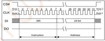
Figure 7.35a Individual Block/Sector Unlock Instruction(SPI Mode)
