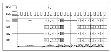
Figure 7.40 Read Manufacturer/Device ID Quad I/O Instruction
