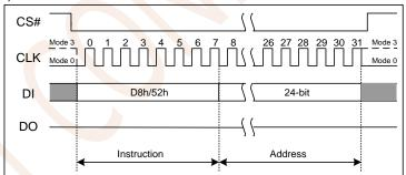
Figure 7.9a Block Erase Instruction(SPI Mode)
