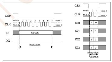
Figure 7.24 Software Reset Instruction(SPI and QPI Mode)
