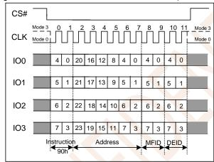
Figure 7.28b Read Manufacturer/Device ID(QPI Mode)
