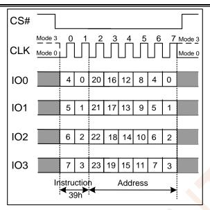
Figure 7.35b Individual Block/Sector Unlock Instruction(QPI Mode)
