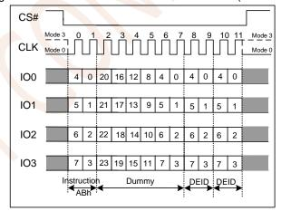
Figure 7.27b Release Power-down / Device ID(QPI Mode)
