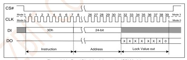
Figure 7.36a Read Block Lock Instruction(SPI Mode)
