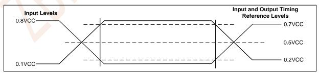
Figure 8.3 AC Measurement I/O Waveform
