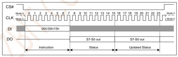
Figure 7.1a Read Status Register Instruction(SPI Mode)
