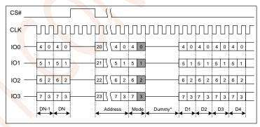
Figure 7.20b Fast Read Quad I/O Instruction(Previous command set M5-4 = 10)
