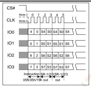
Figure 7.1b Read Status Register Instruction(QPI Mode)
