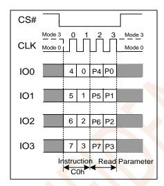
Figure 7.42 Set Read Parameters Instruction (QPI Mode only)
