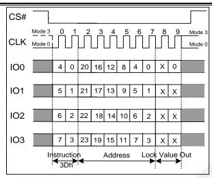
Figure 7.36b Read Block Lock Instruction(QPI Mode)
