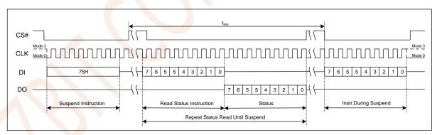
Figure 7.11a Erase / Program Suspend Instruction(SPI Mode)
