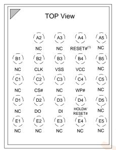
Figure 3.4 24-BALL TFBGA (5x5 ball array)
