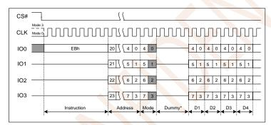
Figure 7.20a Fast Read Quad I/O Instruction(Initial command or previous M5-4 ≠10)
