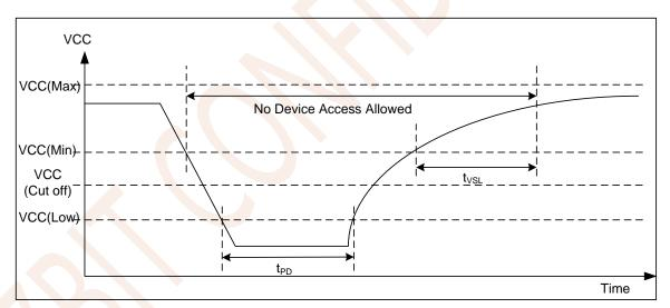
Figure 8.2 Power-Down and Voltage Drop
