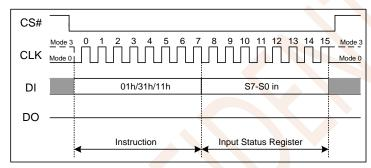
Figure 7.5a Write Status Register Instruction(SPI Mode)
