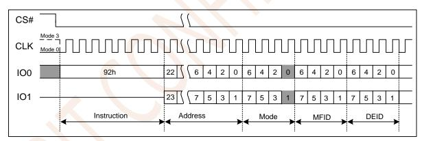
Figure 7.39 Read Manufacturer/Device ID Dual I/O Instruction
