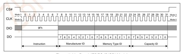
Figure 7.29a Read JEDEC ID(SPI Mode)
