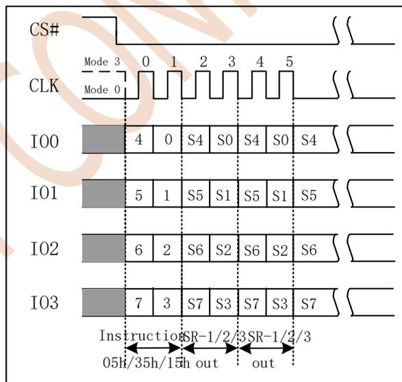
Figure 7.1b Read Status Register Instruction (QPI Mode)
