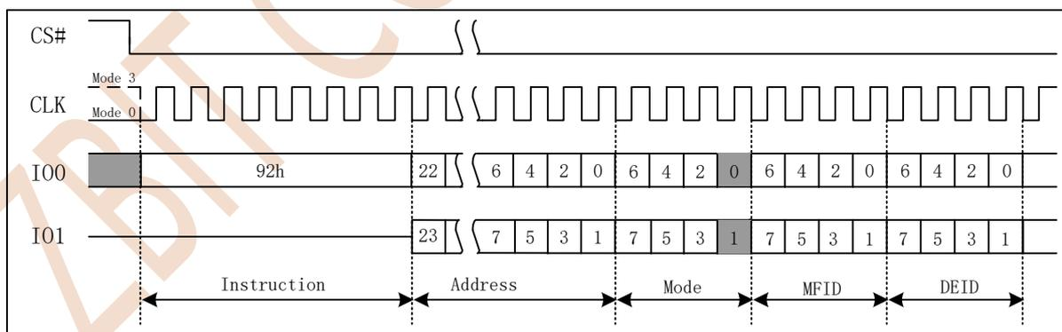
Figure 7.41 Read Manufacturer/Device ID Dual I/O Instruction
