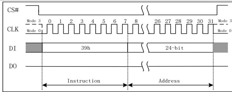
Figure 7.37a Individual Block/Sector Unlock Instruction (SPI Mode)
