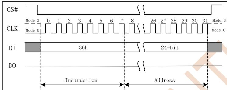
Figure 7.36a Individual Block/Sector Lock Instruction (SPI Mode)
